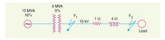
5. What is the fault level? Consider the system shown in Fig below, The percentage of reactance each alternator is expressed on its own capacity determine the short circuit current that will flow into a dead 3 – Ø short circuit at F.
